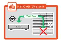
A proportion of FOS NVRs will be assigned as failover servers to the whole surveillance system. Usually 1 FOS NVR shall be worked with 7 NVRs. When any of the NVRs is down, the FOS NVR will soon take over all the works the NVR was doing to keep the whole system working properly. Users could be notified of this take-over event by checking the health check on CMS, and take necessary actions.
